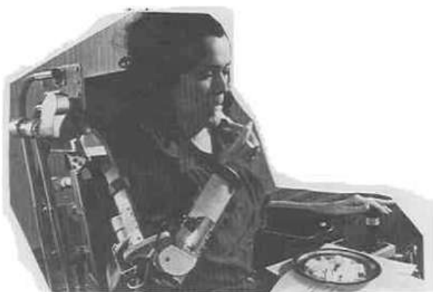
Figure 13. Successfully developed active arm orthosis for the rehabilitation of advanced cases of dystrophy and similar diseases. Controlled by means of a joystick. Made at the Mihailo Pupin Institute in 1982.
